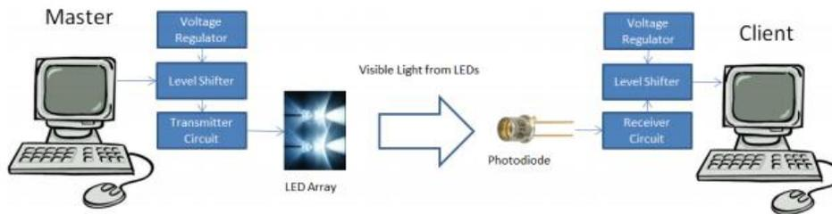
Figure 3: Design of Prototype with USB interface.
