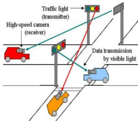
Figure 6 Road-to-Vehicle and Using High Speed Cameras
