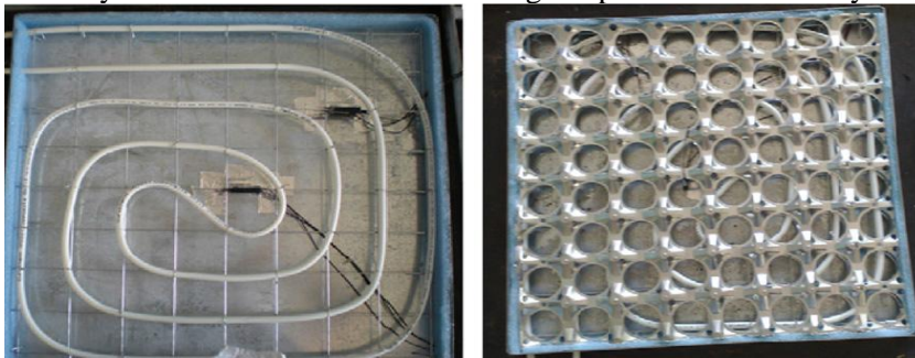
Figure 16: PCM based radiant floor experimental set-up (Ansuini et al. 2011)
